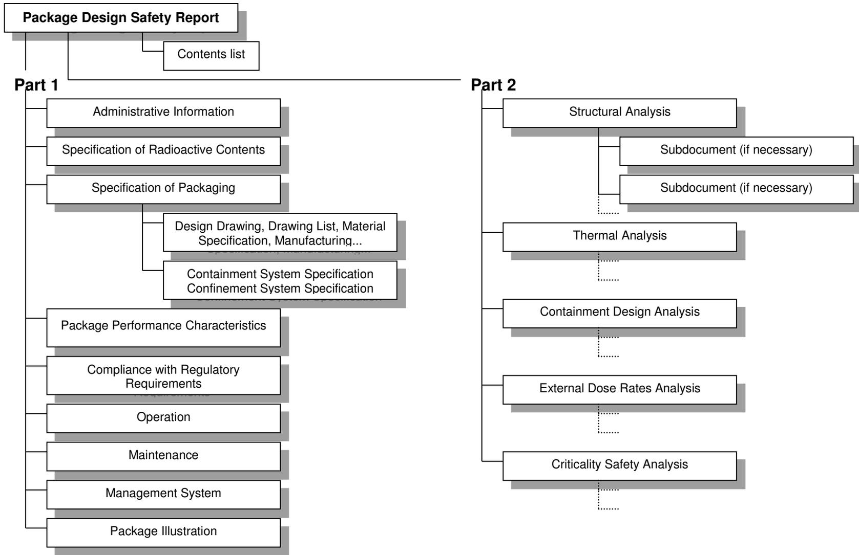
FIGURE 1: Structure of Package Design Safety Report
