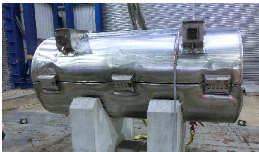
Figure 62: Sequence 4 - Deformation after the 9.0 m drop
