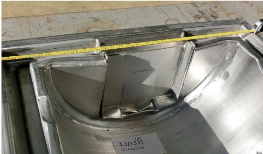
Figure 38: Sequence 1 – Deformation and cracks of the top half, inner shell
