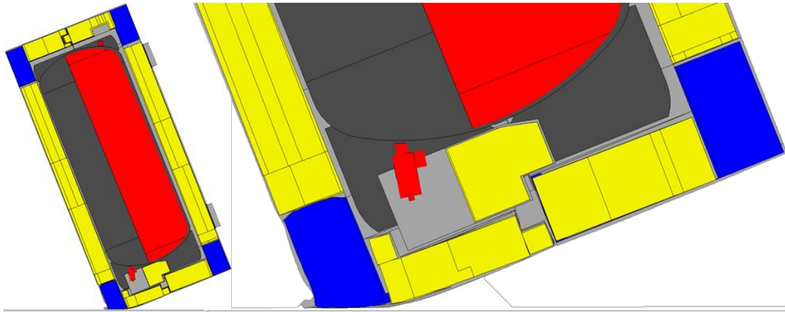
Figure 30: Deformed structure after the 1.2 m free drop onto the valve corner
