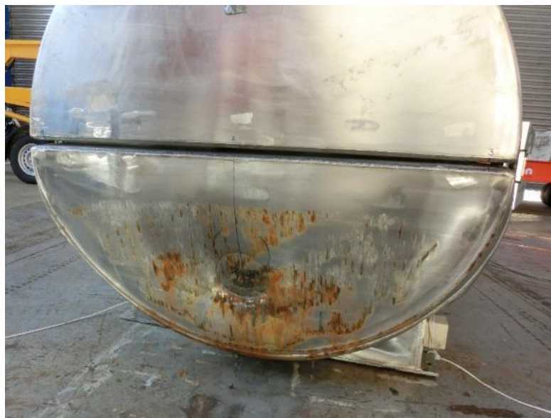
Figure 47: Sequence 2 - Deformation after the drop onto a bar from 1.0 m
