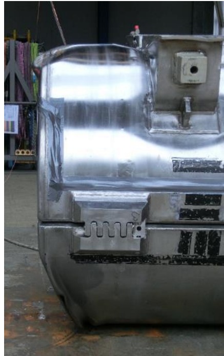
Figure 36: Sequence 1 - Deformation after the 9.0 m drop
