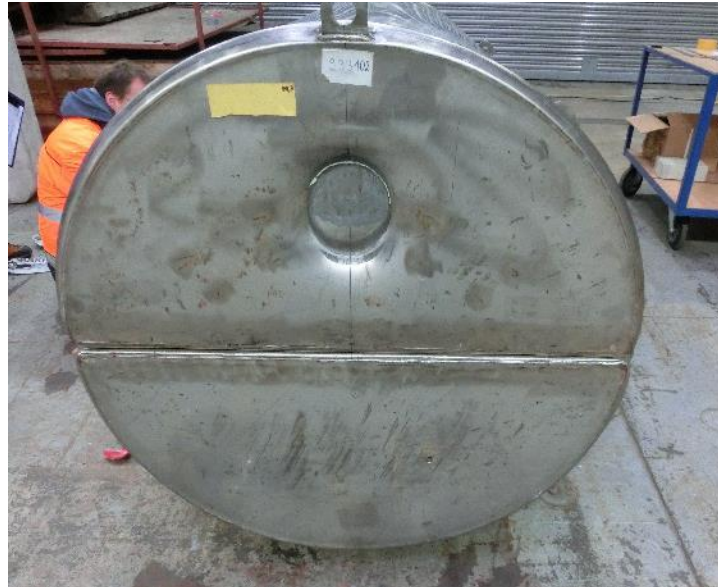
Figure 56: Sequence 3 - Deformation after the drop onto a bar from 1.0 m
