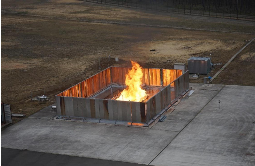
Figure 88: Picture of the fire test showing the full flame engulfment of the DN30 prototype
