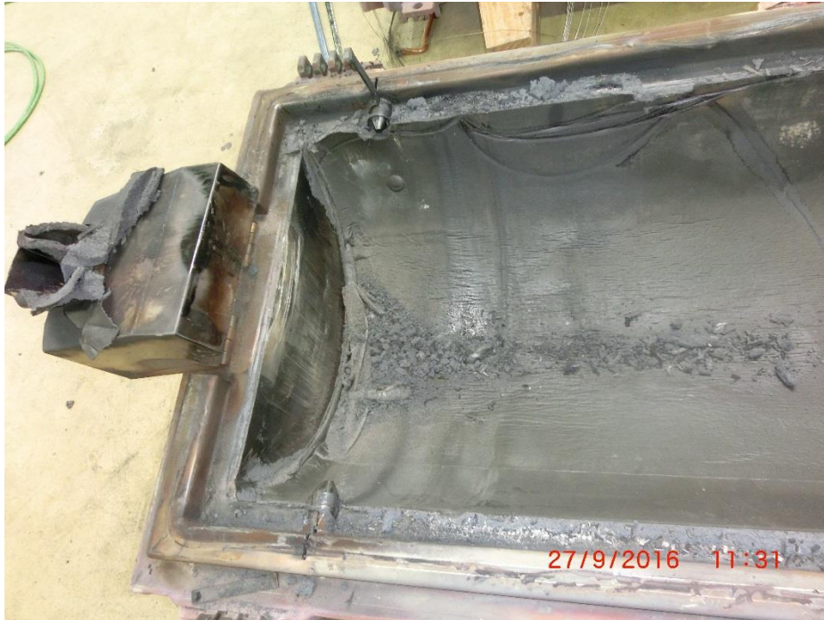
Figure 92: Expanded intumescent material inside the bottom half of the DN30 PSP
