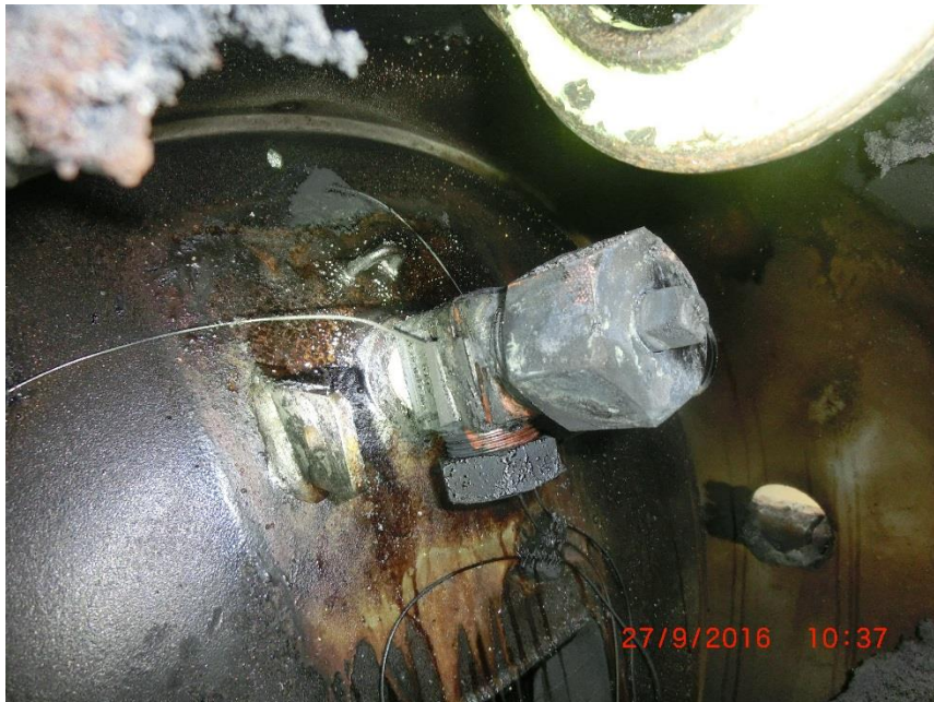
Figure 93: 30B cylinder valve after the thermal test
