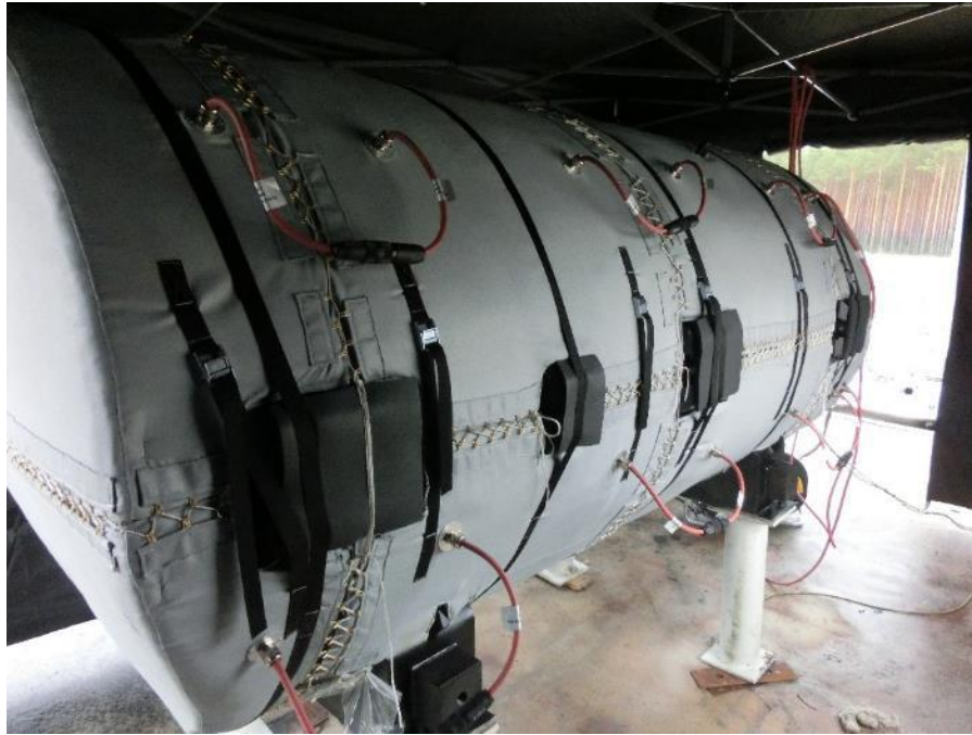
Figure 87: DN30 prototype in heating jacket
