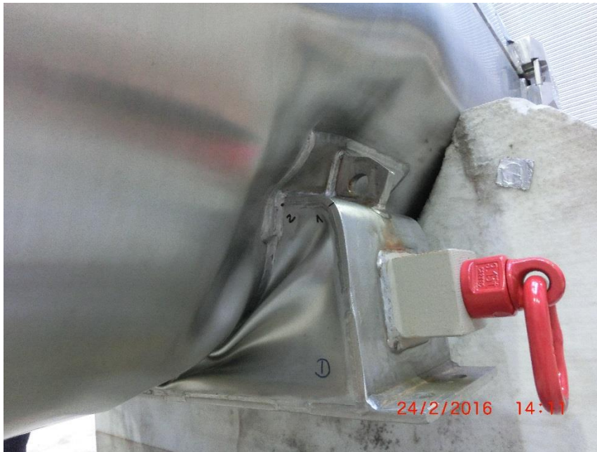
Figure 73: Sequence 5 - Deformation after the 9.0 m drop
