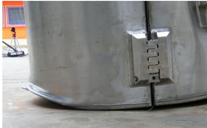
Figure 35: Sequence 1 - Deformation after the 1.2 m drop
