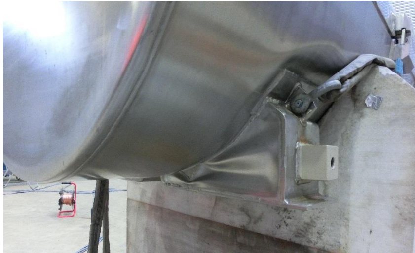
Figure 72: Sequence 5 - Deformation after the 1.2 m drop
