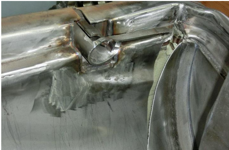
Figure 57: Sequence 3 – Deformation of the bottom half, inner shell
