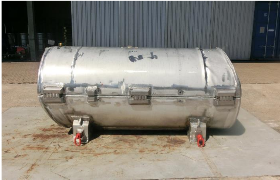
Figure 84: Thermal test prototype after drop test sequence 7
