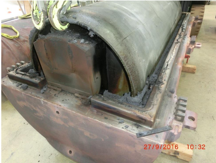
Figure 90: 30B cylinder inside the DN30 PSP after the thermal test
