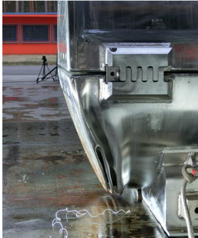
Figure 46: Sequence 2 - Deformation after the 9.0 m drop
