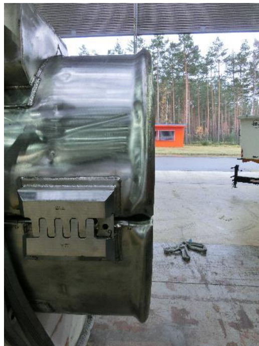
Figure 55: Sequence 3 - Deformation after the 9.0 m drop
