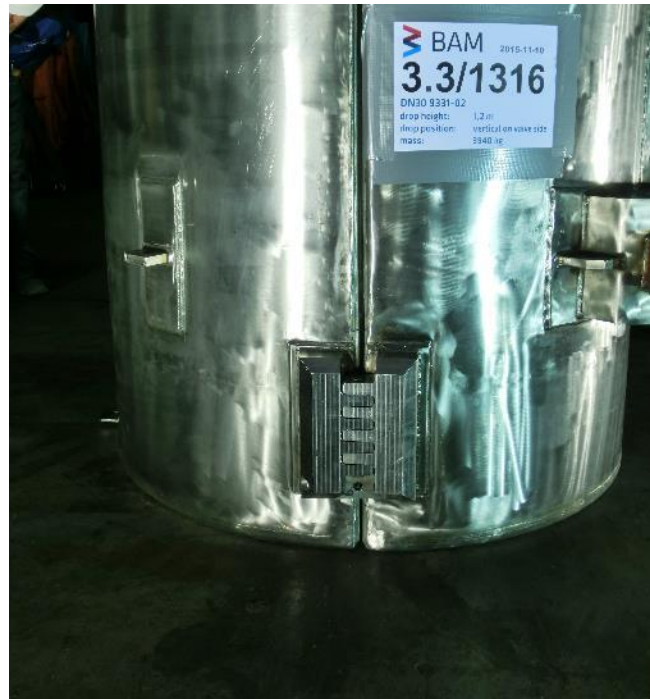
Figure 54: Sequence 3 - Deformation after the 1.2 m drop
