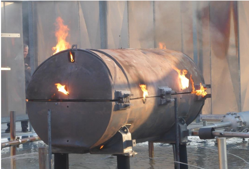
Figure 89: Gases escaping from the DN30 prototype during the cooling phase
