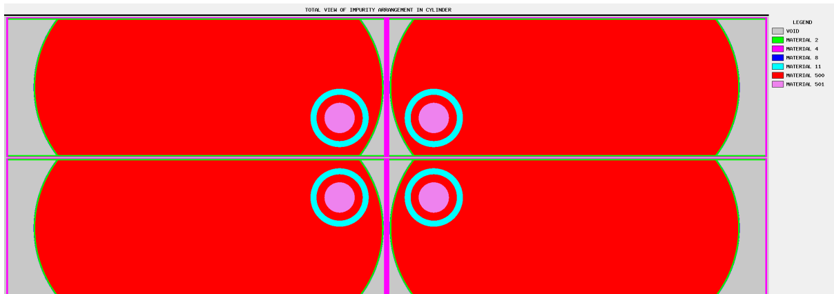
Figure 108: Cross section of the arrangement of two cylinders with impurity sphere for corner-to-corner orientation (plane through center of spherical arrangements)
