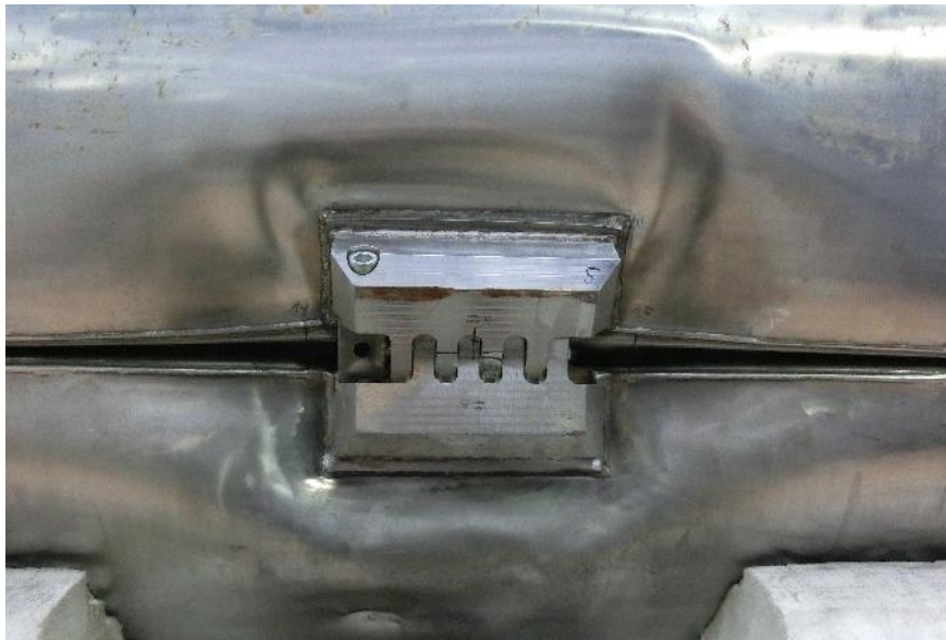
Figure 63: Sequence 4 - Deformation after the drop onto a bar from 1.0 m
