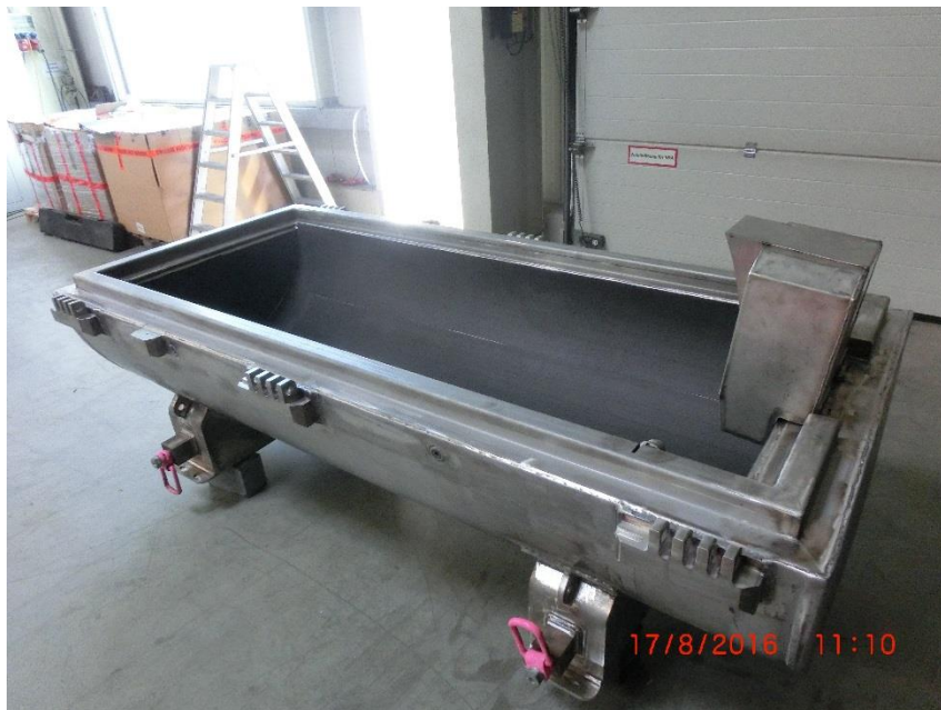
Figure 85: Bottom half of the DN30 PSP before the thermal test
