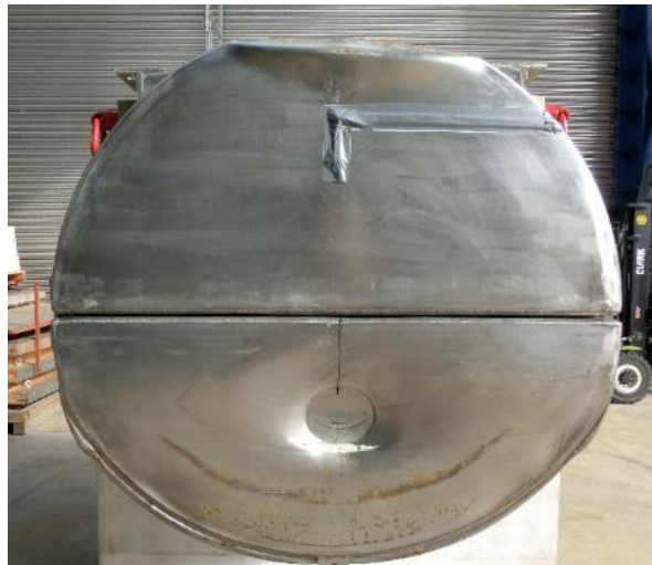
Figure 37: Sequence 1 - Deformation after the drop onto a bar from 1.0 m
