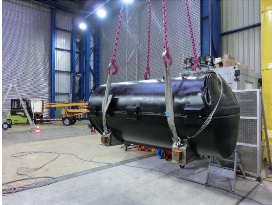
Figure 86: DN30 prototype coated for the thermal test
