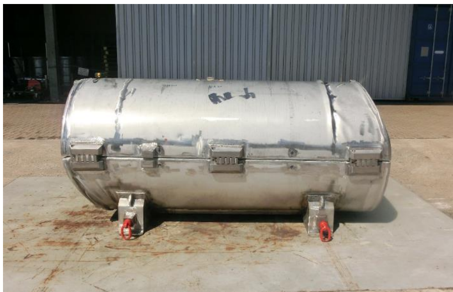
Figure 40: Deformations of the DN30 PSP after sequence 7
