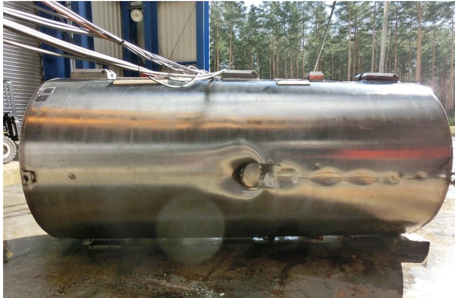
Figure 74: Sequence 5 - Deformation after the drop onto a bar from 1.0 m
