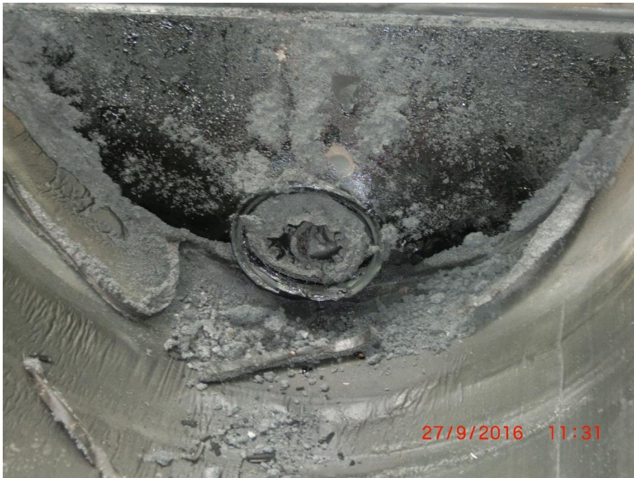
Figure 91: Expanded intumescent material inside the plug protecting device
