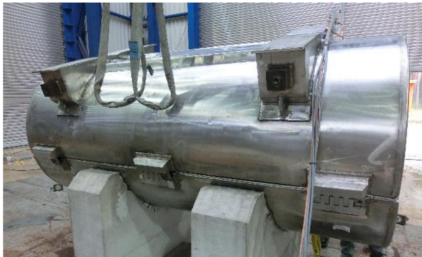
Figure 61: Sequence 4 - Deformation after the 1.2 m drop
