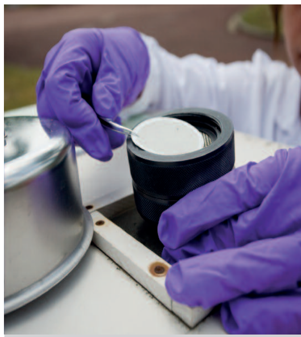
Installing a filter on one of IRSN's "OPERA AIR" aerosol sampling network stations (OPERA programme: permanent environmental radioactivity observatories)
