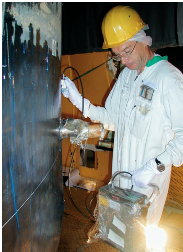
Ultrasonic inspection of a weld joint
