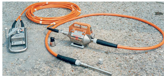
Gamma radiography projector - CEGELEC - and accessories (remote control, ejector tube, irradiation endpiece)
