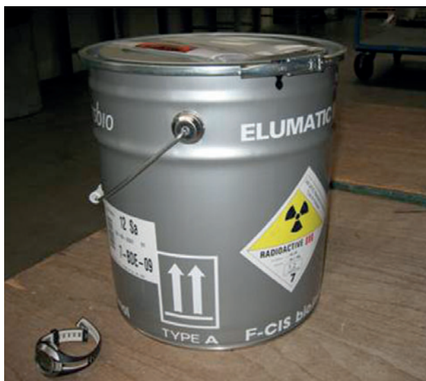
Example of a Type A package – technetium 99m generator
