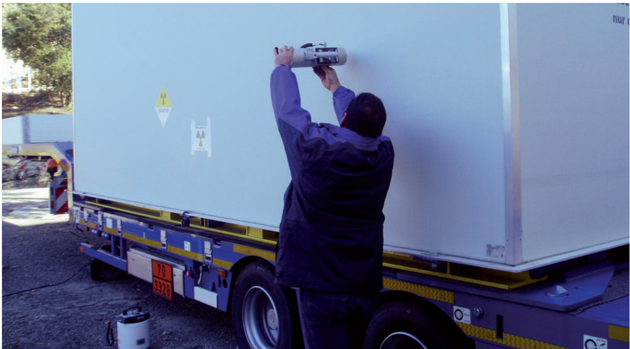
Measuring radioactivity at Cadarache before a spent fuel convoy departs for the Greifswald centre in Germany – December 2010
