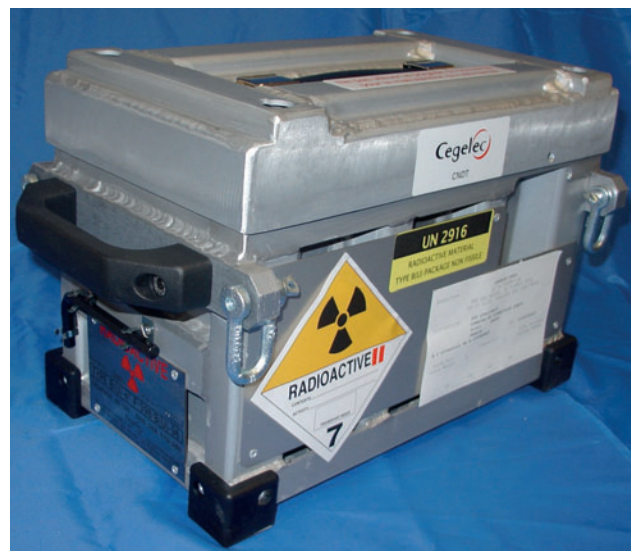
Example of a Type B packaging – Gammagraph containing an iridium source
