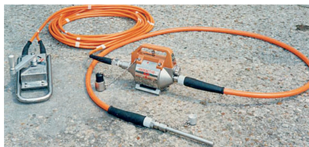
Gamma radiography projector - CEGELEEC - and accessories (remote control, ejector tube, irradiation endpiece)
