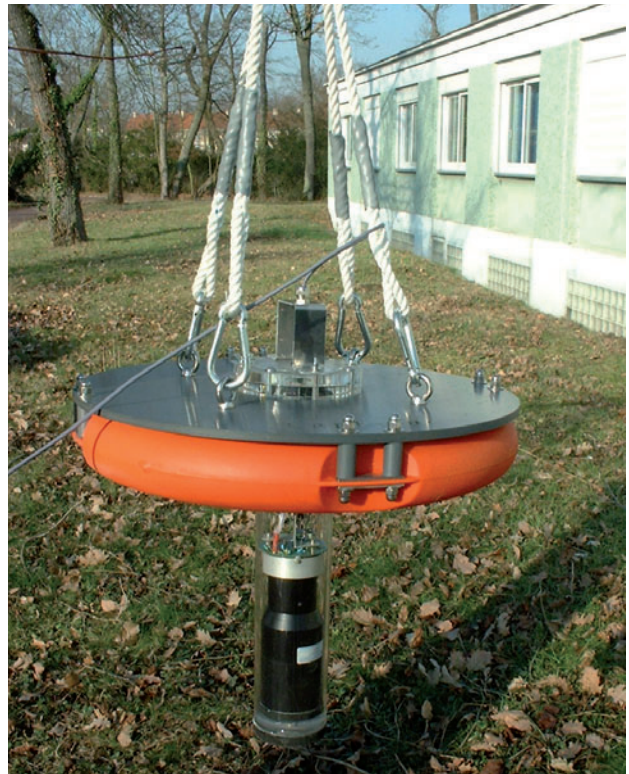
Set-up for measuring wastewater radioactivity
