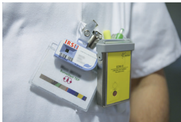
Dosimeter worn by medical personnel in the nuclear medicine unit of the North Saint-Denis Cardiology Centre
