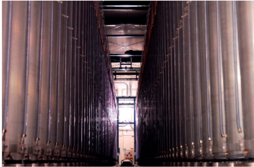
Cascade of centrifuges in the GBII facility on the Tricastin site (Drôme département)
