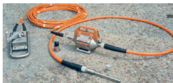
Gamma radiography device – CEGELEC – and its accessories (remote control, ejector tube, irradiation end-piece)
