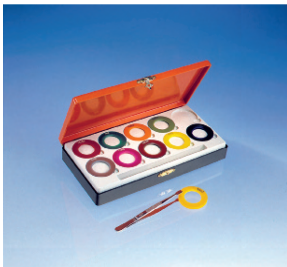
Box of gamma sources manufactured in the LEA. The radionuclides proposed are Am241, Cd109, Ce139, Co57, Cr51, Cs137, Mn54, Sn113, Sr85, Zn65
