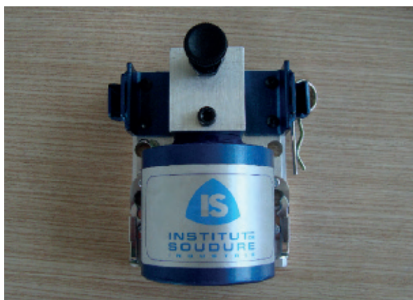
The \gamma -prox (collimator) device developed by the Institut de Soudure and complementing existing gamma radiography devices, is used to optimise radiation protection
