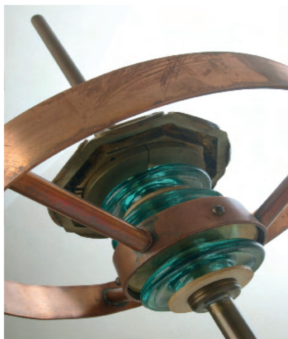
Top of a radioactive lightning conductor
