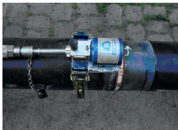
The \gamma -prox (collimator) on a site
