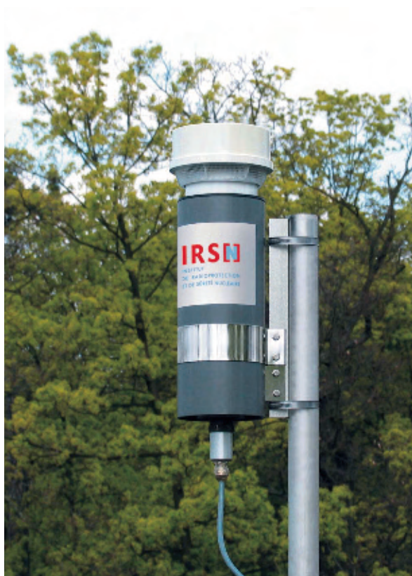
Téléray monitoring network: device continuously measuring ambient gamma radioactivity in the air
