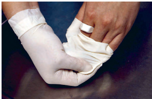
Thermoluminescent ring for personnel radiation protection (measurement of dose at the extremities)
