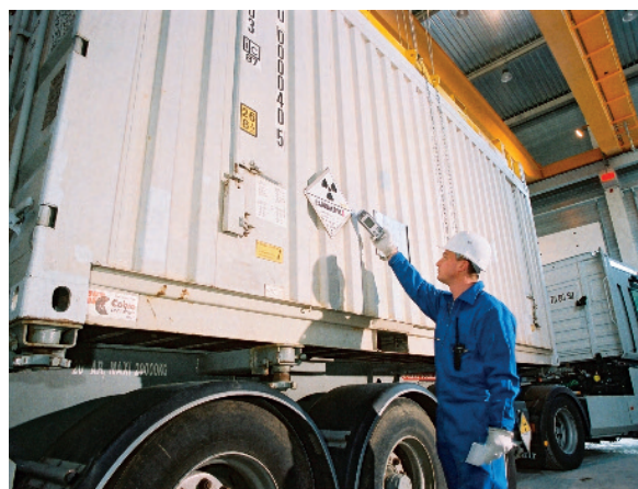
Radiological check on a lorry using a radiation meter in the logistics building of ANDRA's very low level waste repository (CSTFA) in the Aube département – April 2004
