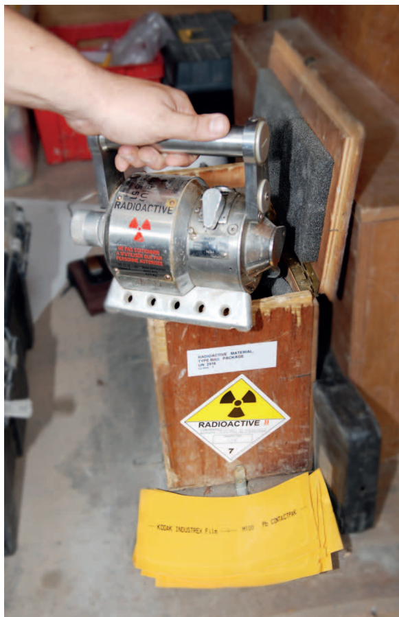
Gamma radiography appliance and its transport case
