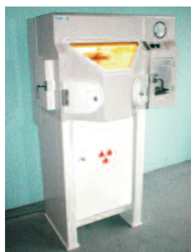
Shielded chamber for handling unsealed radioactive sources
