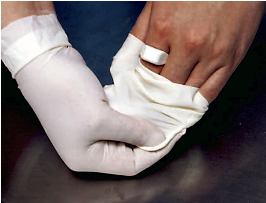
Thermoluminescent ring for staff radiation protection (dose measurement at the extremities)
