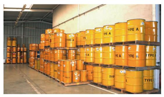
Interim storage of low-level waste packaged in metal drums pending reprocessing (CEA/Saclay)
