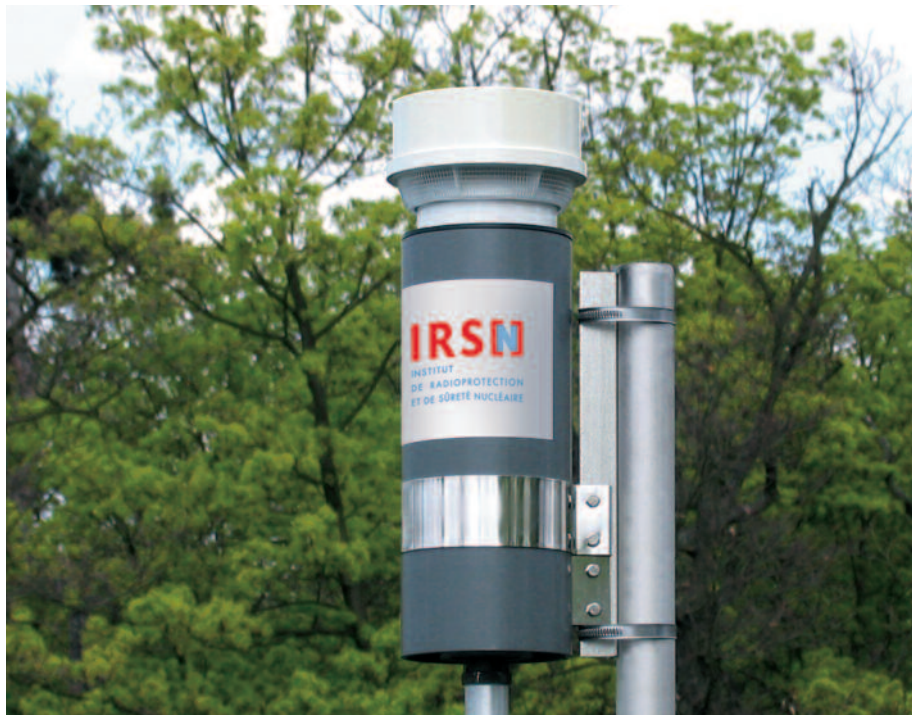
TELERAY radiation monitor for surveillance of the ambient dose rate
