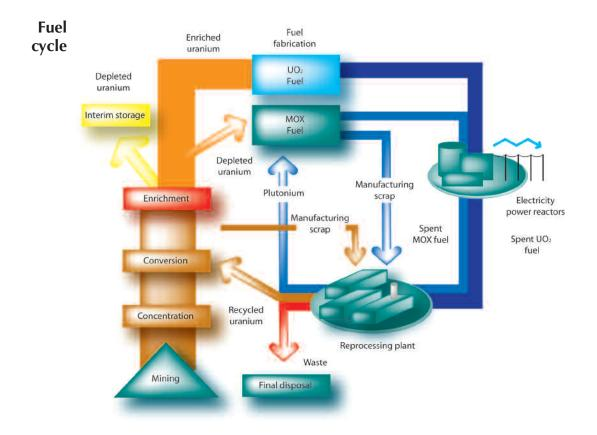
Manufacture of the fuel and its subsequent reprocessing after it has passed through the nuclear reactors constitute the fuel cycle. The cycle begins with extraction of the uranium ore and ends with disposal of a range of radioactive waste streams arising from the spent fuel.
