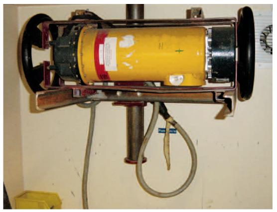
Electric X-ray generator in a radiography chamber
