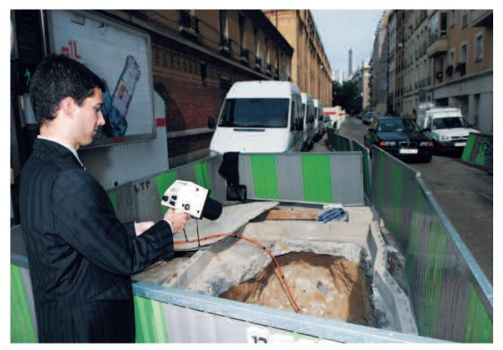
Dose rate measurement before a gammagraphy operation
