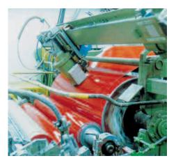
Basis weight measurement by backscatter
