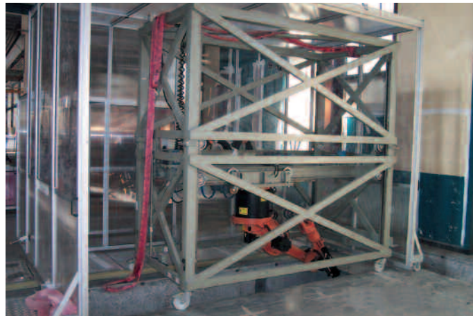
Adjustment of a bush hammering robot (pilot worksite) – SICN
