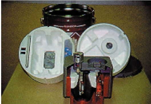
Example of a type A packaging – Technetium 99 generator
