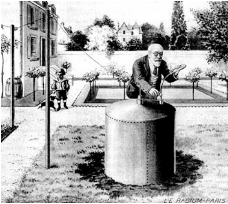
Ancestor of radon flux measurement in the soil using an accumulation chamber
