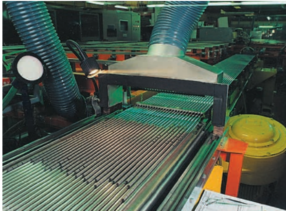
FBFC – pellet incorporation into fuel rods
