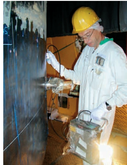
Ultrasound inspection of a welded joint
