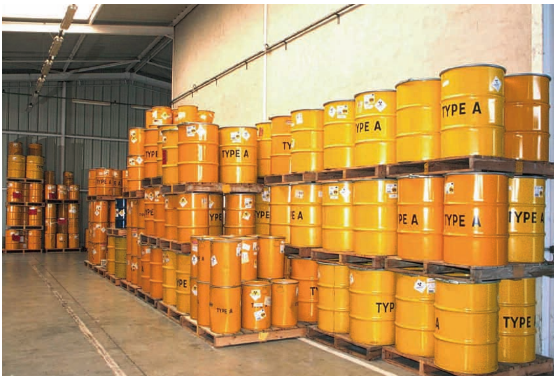
Interim storage of low-level waste packaged in metal drums pending reprocessing (CEA/Saclay)
