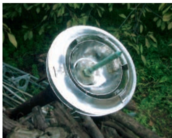
Radioactive lightning conductor
