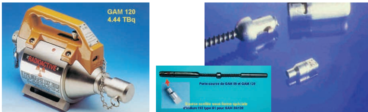
Gammagraphy equipment and its radioactive source
