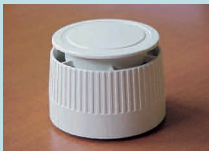
Smoke detector with its radioactive source
