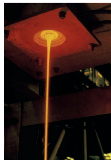
Vitrification of a solution of fission and activation products
