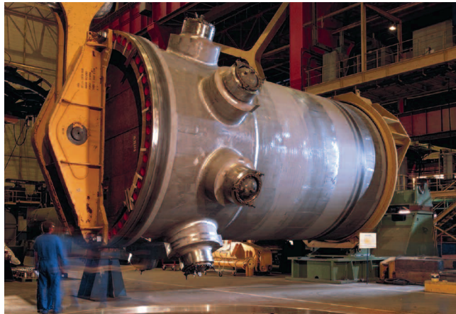
Vessel being manufactured
