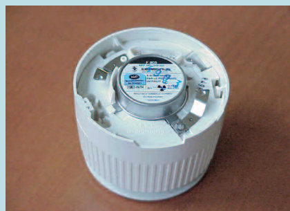
Smoke detector with its radioactive source
