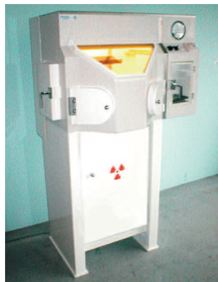
Shielded chamber for handling unsealed radioactive sources
