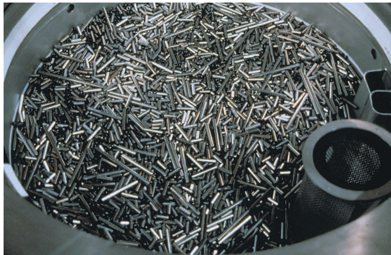
Fuel assembly hulls, COGEMA La Hague ACC shop
