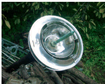
Radioactive lightning conductor
